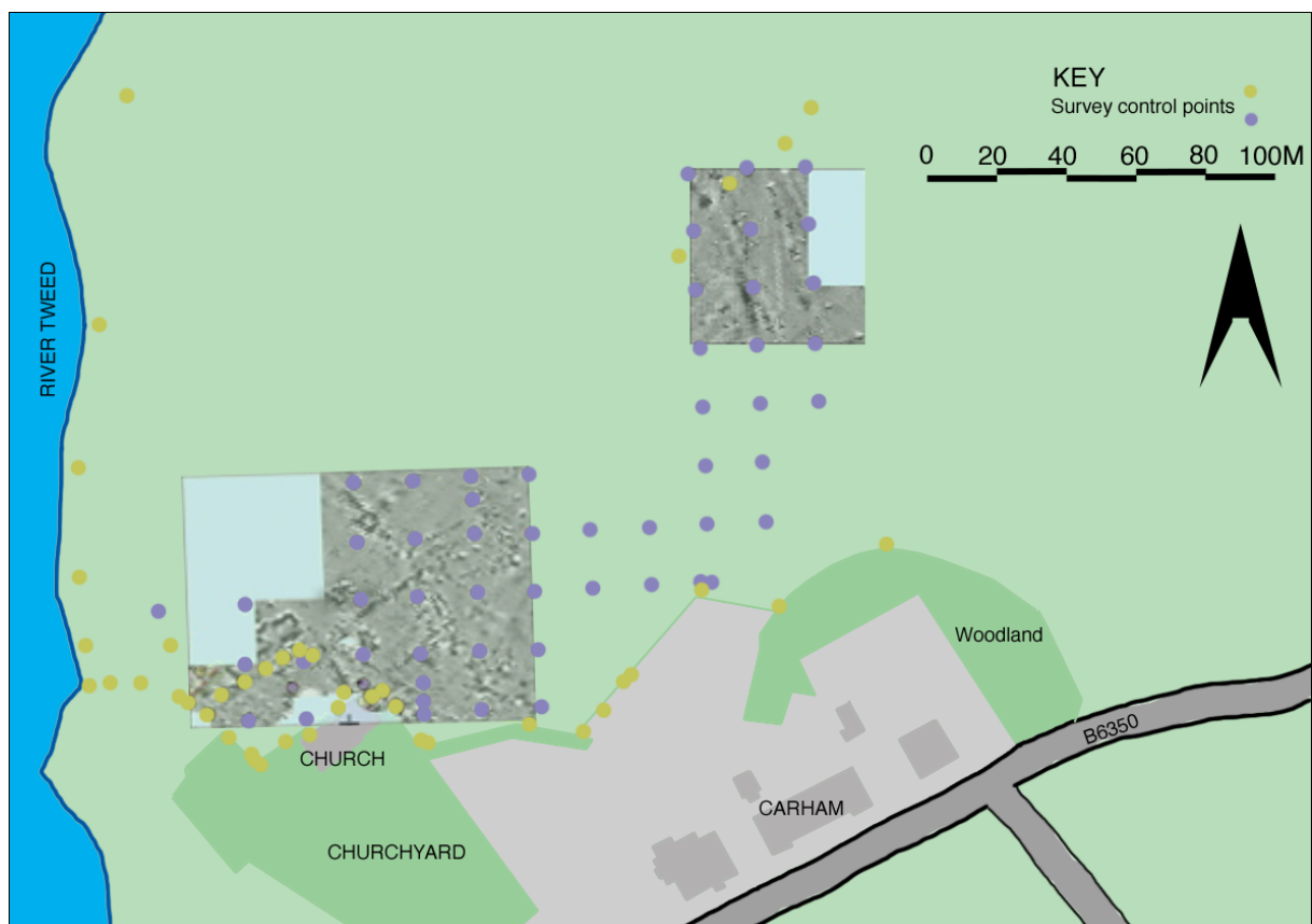
Figure 6.2: Overlay Map showing Carham, grid marker pegs, topographical features and the East and West survey sites
